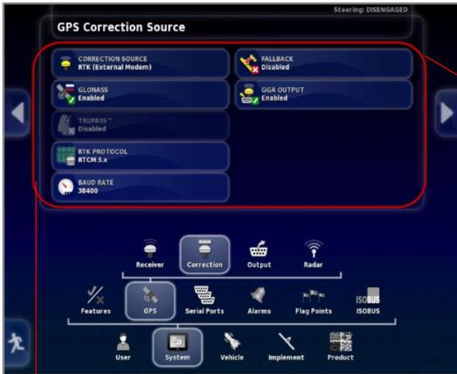
5 Configure the GPS correction source page according to the shown settings
