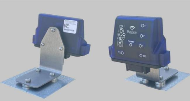
1. Use 3 screws supplied with kit and attach Beacon 4 to tapered part of bracket. Don't overtighten.
