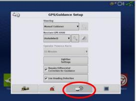
5 Enter the GPS/Guidance Setup menu by pressing the receiver and wheel icon at the bottom
