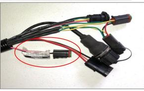
Connect the Power Tee to the Can B power / Terminator connection on the Display cable
