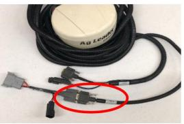
1 Connect the Elevate and the adapter to the **Port B** connection on the Ag Leader 6500/7500 cabling
