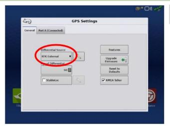
7 Ensure the Differential source is set to "RTK external"
