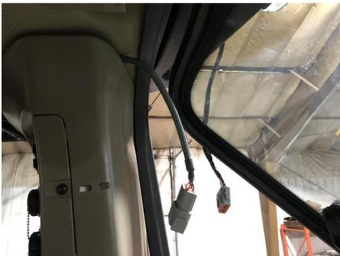
8 Re-attach corner plastic with cable routed as shown.
