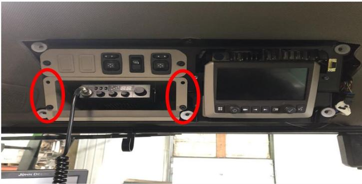
2 Use Torx 30 to remove (4) screws. Pull out the entire insert.
