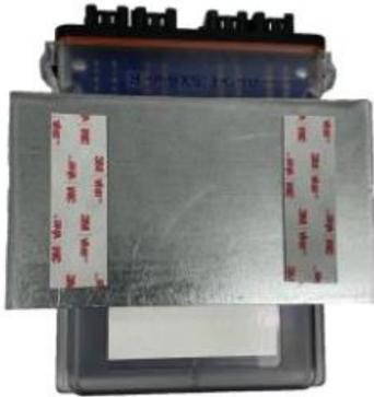
10 Use the included alcohol swabs to clean the mounting area. Peel back the sticker tabs and press the mounting plate firm on the cleaned cab roof.
