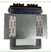
Use the included alcohol swabs to clean the mounting area. Peal back the sticker tabs and press the mounting plate firm on the cleaned cab roof.
