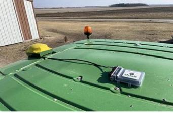
Run the long end of the cable to the roof and plug into the modem in port A.
