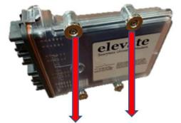
4 Place elevate slim on the installed mounting plate with the magnets facing down.
