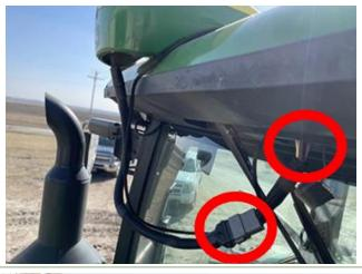
1 Unplug the receiver cable from under the cab. Plug-in in T-cable to the male connector on cab and female end to receiver.
