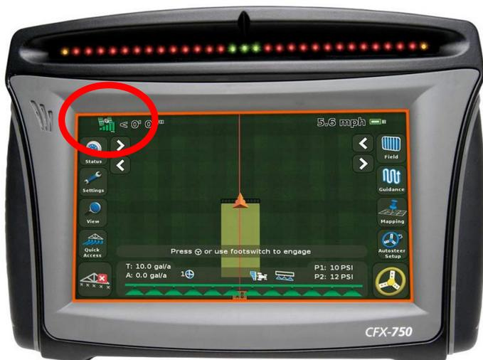
11 Confirm RTK by returning to the mapping screen and confirming a green satellite icon in the top left corner.
