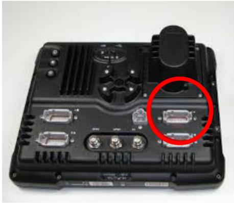
1 Install the Elevate cable into the EXP-100 port expander cable
