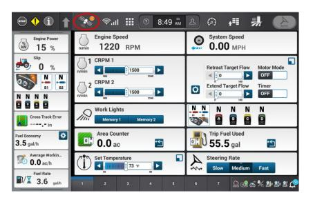
Return to the GNSS & Guidance and confirm RTK fix with the **Green Satellite Icon** in the top left corner.
