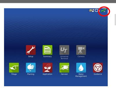
Confirm RTK fix by returning to the home screen and confirming the satellite has gone green
