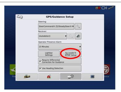
From the GPS/Guidance Set Up screen, select 'Ag Leader NTRIP Setup'
