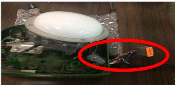
6 Plug into antenna base & plug Deere connector into cable.
