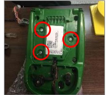
3 Remove 3 screws to detach antenna from shroud.
