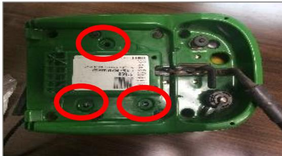
4 Lift antenna from shroud to expose main connector & unplug it.
