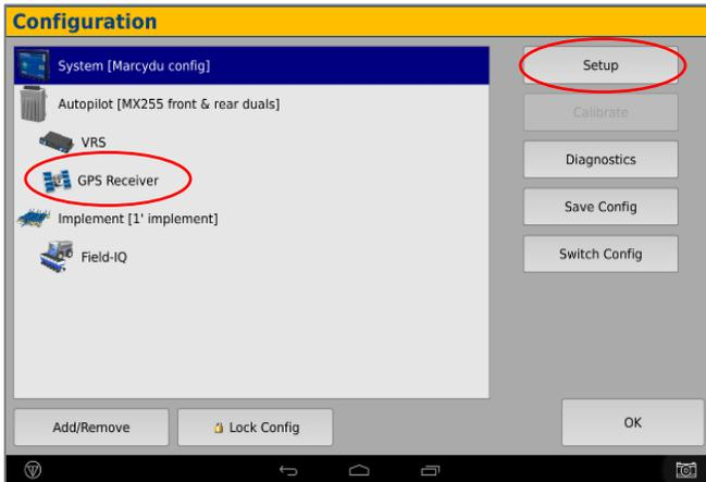
4 On the GPS setup page change the Corrections to Centerpoint RTK
