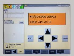
Program Port C of the receiver on the RDI screen: Right arrow twice to configuration>Down arrow to Config menu>Right arrow to Port C config>Down arrow to enter> Verify Port C Flow is on & Port B flow is off> Down arrow once to next screen.
