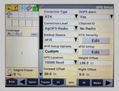
On the GPS setup screen, Set the correction type to RTK, Corrections level to AGGPS Radio. Enable the the backup source to xFill, set xFill options to custom>select xFill Setup Edit.
