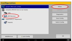
On the GPS setup page change the Corrections to CenterPoint RTK
