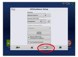
Ensure the Differential source is set to "RTK external"
