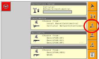
4 Select Cellular Network; checkmark "Use external radio"; then select the checkmark on the right
