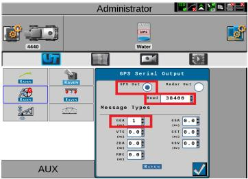
Select RTK Source and set to serial and 38400 Baud
