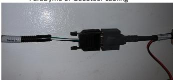
Connect the Power Tee to the Can B power/ Terminator connection on the Display cable
