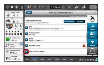
Create a new output configuration. Turn Terrain compensation off (this is only for the output, this does not impact the terrain compensation for the steering system). Set your port selection to Receiver Serial Port #1. Turn Port on. Set Baud rate to 38400. Select GGA, Turn it on, se the rate to 1
