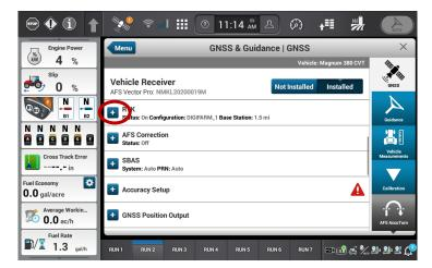
Turn RTK on, Set a new configuration and name. Set the Correction source to RTK External Device. Port setting: Receiver serial port #2. Data parity: None. Baud rate:38400. Stop bits 1. Protocol RTCM 3.
