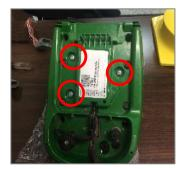
Lift antenna from shroud to expose main connector & unplug it.
