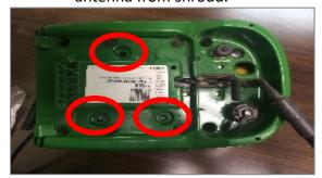
Reassemble the receiver so the smart cable routes through the square hole in the rear of the shroud.
