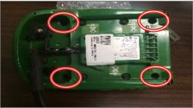
Remove 3 screws to detach antenna from shroud.
