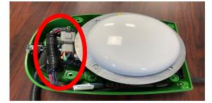
8 Reinstall 3 screws & removed decals. Attach shroud.
