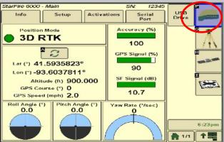
Go to the serial port page & confirm: 11 Baud Rate is 38400, Output rate at 1Hz & GGA box check marked.
