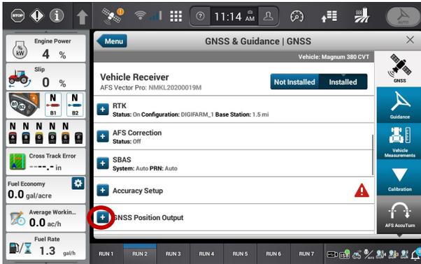
6 Create a new output configuration. Turn Terrain compensation off (this is only for the output, this does not impact the terrain compensation for the steering system). Set your port selection to Receiver Serial Port #1. Turn Port on. Set Baud rate to 38400. Select GGA, Turn it on, set the rate to 1
