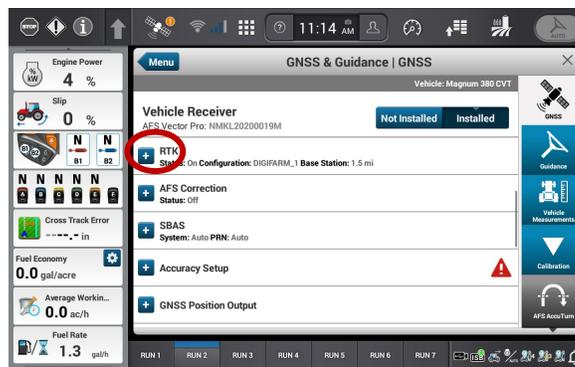
4 Turn RTK on, Set a new configuration and name. Set the Correction source to RTK External Device. Port setting: Receiver serial port #2. Data parity: None. Baud rate:38400. Stop bits 1. Protocol RTCM 3.
