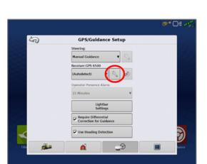
5 Ensure the Differential source is set to "RTK external"
