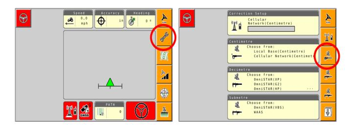
Select Cellular Network; checkmark "Use external radio"; then select the checkmark on the right
