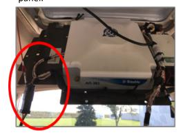
**Note:** Placement of the elevate modem on the cab roof is vitally important to performance. User must extend the entire length of the cable away from the receiver as shown below. **DO NOT MOUNT THE ELEVATE DIRECTLY ABOVE THE IN ROOF RECEIVER**
