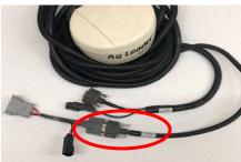
Connect the Power Tee to the Can B power/ terminator connection on the Display cable
