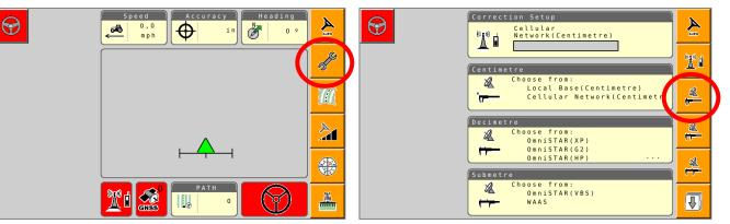
4 Select Cellular Network; checkmark "Use external radio"; then select the checkmark on the right
