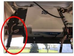
**Note:** Placement of the elevate modem on the cab roof is vitally important to performance. User must extend the entire length of the cable away from the receiver as shown below. **DO NOT MOUNT THE ELEVATE DIRECTLY ABOVE THE IN ROOF RECEIVER**
