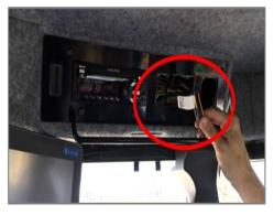
2 On the Fendt & Challenger series, it is located on the VDO3 to receiver cabling above the drop-down roof panel.
