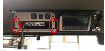
1). Plug "T" Cable here. 2). Plug original JD cable here. 3). 47" end going back toward B post.
