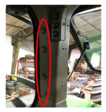
Re-attach corner plastic with cable routed as shown.
