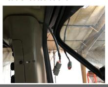
Use Torx 30 to remove (4) screws. Pull out the entire insert.
