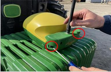
2 Pull the radio away from the receiver. Unplug the radio cable.
