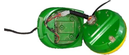
9 Gently set antenna base on shroud. Re-install the base screws.
