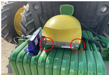
11 Place the receiver onto roof mount and plug in the receiver to the cab.
