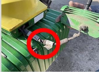
3 Place the orange dust cap onto the male end of the plug and push cable into receiver.
