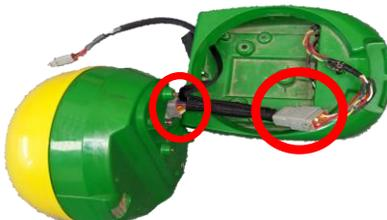
8 Thread the long end of the T cable through the hole in the base.
