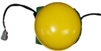
10 Use the 3 screws included in your Beacon 4.0 kit and attach to bracket. Screw bracket on receiver with the 2 screws removed from radio un-installation.
