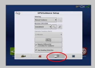
From the GPS/Guidance setup screen, select the wrench icon next to "Autodetect"
