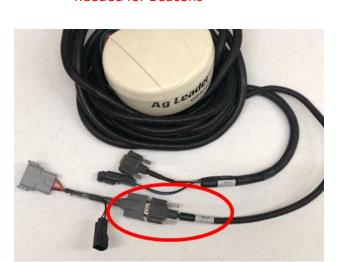
Connect the Power Tee to the Can B power/ terminator connection on the Display cable
