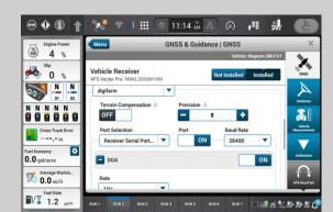
9 Select the satellite icon from the top bar and confirm RTK fix.
