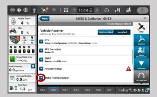
Create a new output configuration. Turn Terrain compensation off (this is only for the output, this does not impact the terrain compensation for the steering system). Set your port selection to Receiver Serial Port #1. Turn Port on. Set Baud rate to 38400 Select GGA, Turn it on, se the rate to 1
