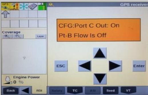
8 Right arrow once to select TSIP>Down arrow to RTCM (CMR for 252/262)>Confirm Baud rate is set to 38K.4> right arrow 5 times to the bottom TSIP>Down arrow to change this to NMEA>Enter (confirm setting with screenshot to the right)
