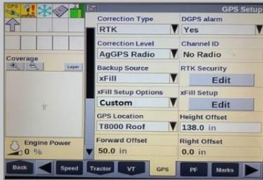
5 On the GPS setup screen, Set the correction type to RTK, Corrections level to AGGPS Radio. Enable the the backup source to xFill, set xFill options to custom>select xFill Setup Edit. Set the custom fields to match the screen to the right
