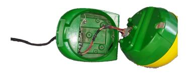
Plug the male end of the T cable into the globe then plug the female end into the connector on the base.
