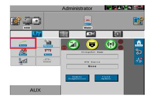
Select RTK Source and set to serial and 38400 Baud
