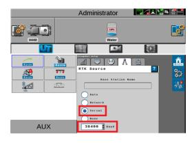
Return to the RS1 UT screen and confirm RTK
