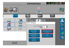
7 Set Differential source to RTK and RTK Format to RTCMV3, then select the checkmark.
